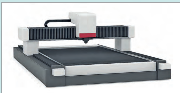
Rack and pinion gears in flatbed lasers – ideal for high cutting speeds and smooth operation.
